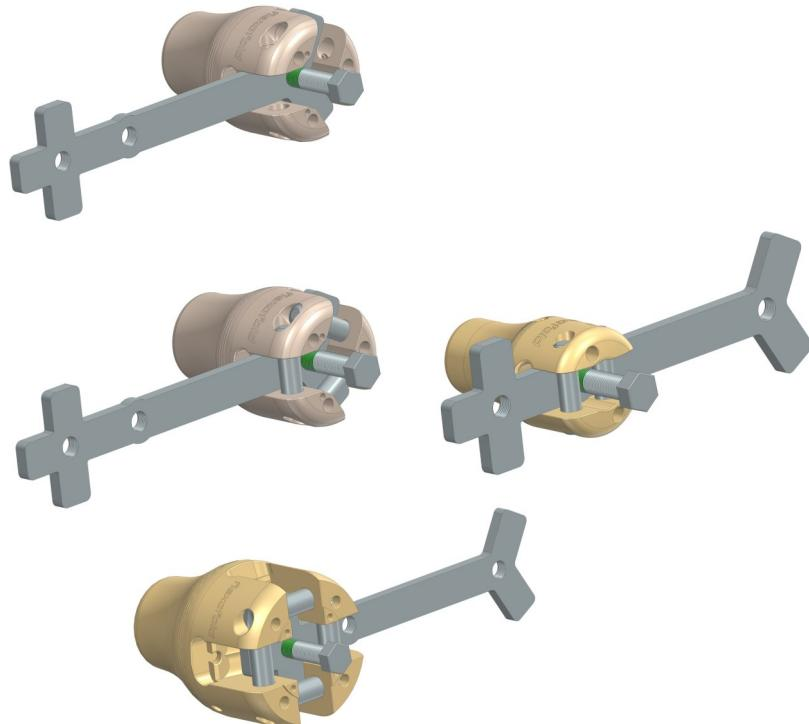
3 Mount ALL the pivot pins and locking screws.
