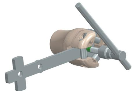
5 If the hub does not move, strike the screw end to apply a shock impact to the hub.
